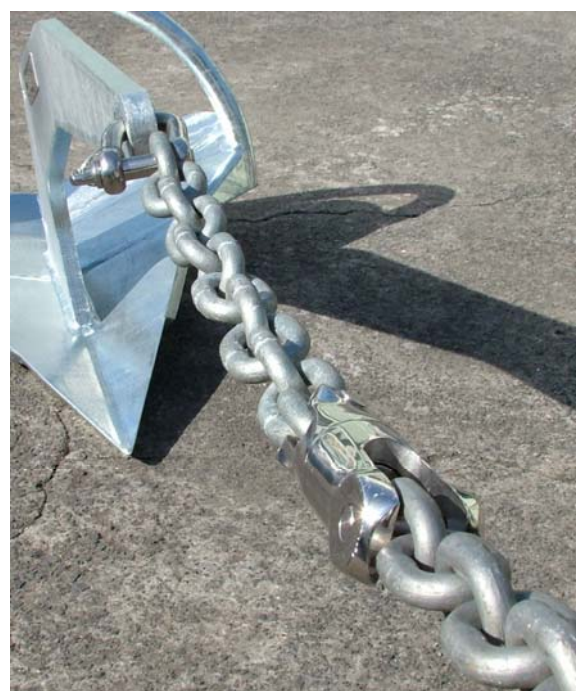
Above: Single shackle between the chain and anchor. Important - always seize the pin Below: Popular inline type swivel installed with a few links of chain between it and the anchor
