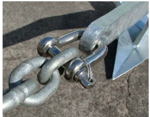
Above: Single shackle between the chain and anchor. Important - always seize the pin Below: Popular inline type swivel installed with a few links of chain between it and the anchor
